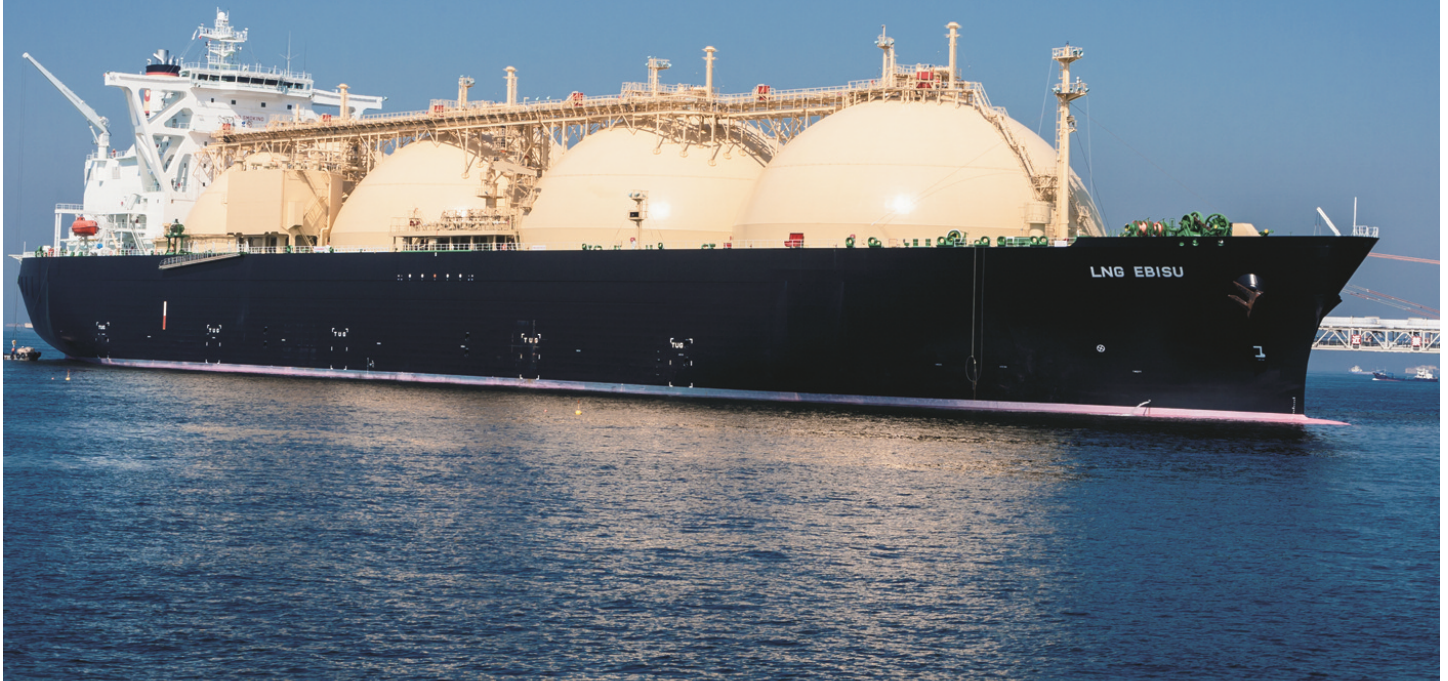
Picture: An LNG carrier, with the characteristic round tanks, for transporting liquefied natural gas.
